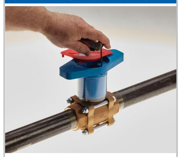
Trim service times with INSULATOR/MS<sup>®</sup>. Unlike other insulating ball valve handles with memory stop, INSULATOR is the only one you can adjust without taking the handle apart. Simply pop off the top cover to make memory stop adjustments with a hex wrench.
