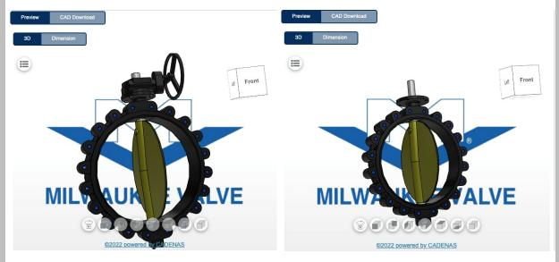
Both high and low-level of part details allows Milwaukee Valve to deliver BIM-friendly downloads to engineers and contractors. These digital renderings contain the accurate part number and the metadata that the contractor needs, without having to build the part with their BIM software. The 3D part catalog features 150+ CAD and BIM formats, including Autodesk REVIT<sup>®</sup>.
