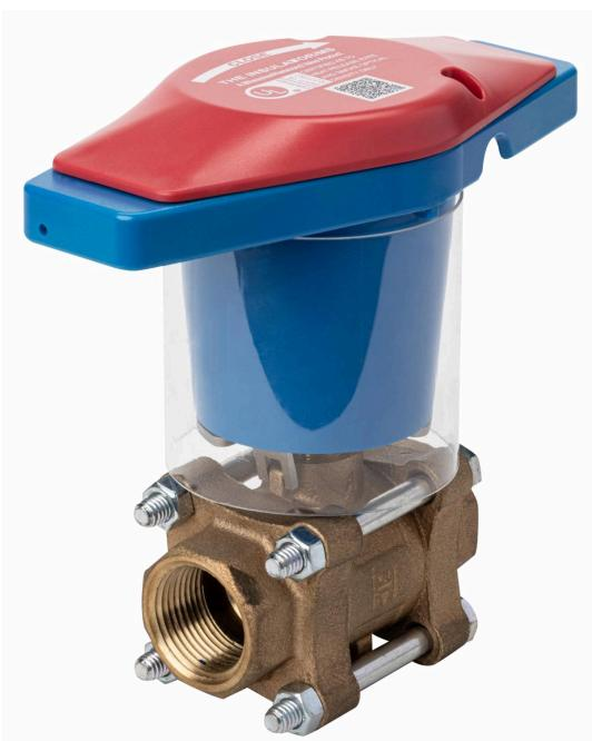
As with the INSULATOR/TIH, **TIHL** creates a heat-transfer barrier between piping systems and the exposed portion of a valve handle and surrounding air. This barrier reduces or eliminates condensation, and keeps damaging moisture from
