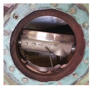
Due to the characteristics of steam, if a disc is positioned less than 30 degrees open, it creates high velocity flow in the area between the disc and the seat. This high velocity steam can pull part of the seat out, which gets crinkled and damaged when the operator tries to close the valve.
