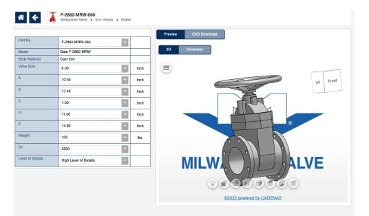
The F-2882-MRW and the F-2885-MRW are flanged ductile-iron valves with epoxy coating and full NSF/ANSI 61 & 372 approvals for domestic/potable water systems. Available in both OS&Y rising stem (2885) and non-rising stem (2882) configurations, the non-rising stem valves are available with either a handwheel or square nut operator. Sizes range from 2-1/2 through 12 inches are rated to 300 psi WWP. The 14-inch and 16-inch sizes are rated to 250 psi WWP for each valve type.
