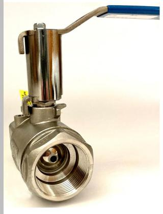
The most widely held understanding of a "vented ball" is one in which a relief hole is drilled in the upstream side of the ball (the Milwaukee Valve –VB option). When the valve is closed, any media inside the valve has a path to "vent" to the upstream piping. Many industrial applications have temperature fluctuations that can cause significant increases in cavity pressure, potentially
