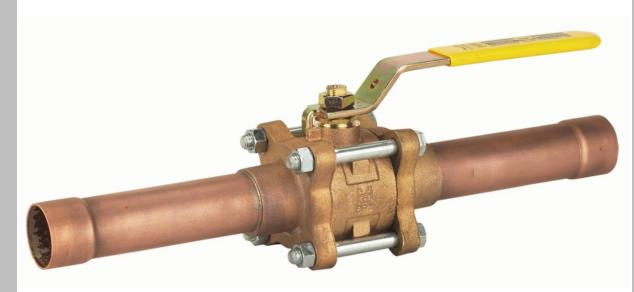
The **BA350TE** is available in sizes ranging from 1/2" – 3". For increased installation flexibility, the **BA350TE** can be ordered with straight male tube-ends, female expanded ends or with a combination of male and female ends. Manufactured and tested in accordance with MSS SP-110, the valve's full-port design provides high flow with minimal pressure drop, and the 3-piece construction simplifies maintenance and repair.
