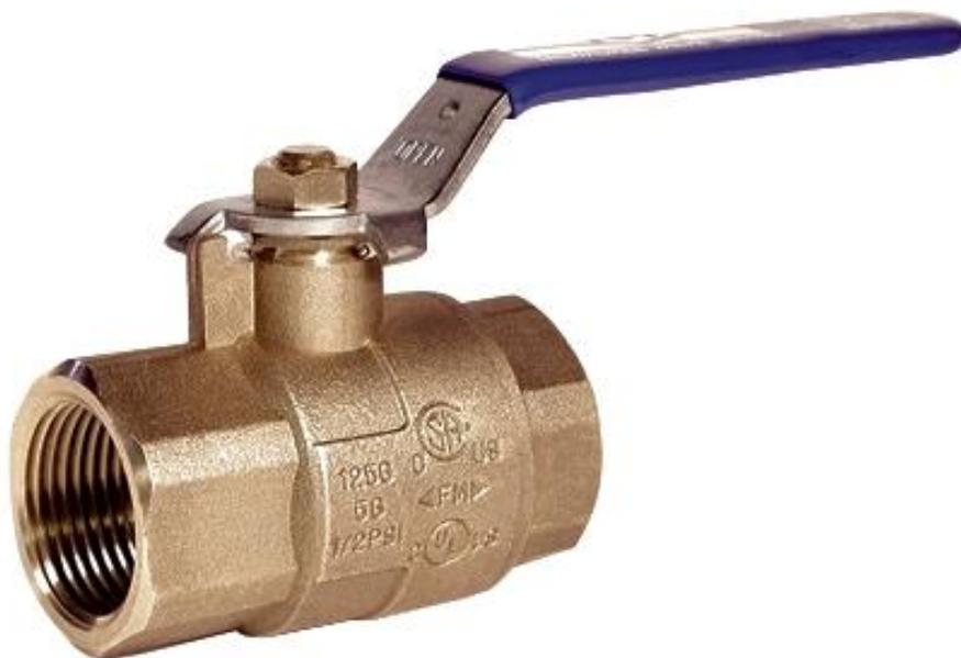
The 5G mark signifies that the valve meets the requirements of [ASME B16.44](#). B16.44 applies to quarter-turn, manually-operated metallic valves, intended for indoor installations as shutoff valves when installed in above-ground, fuel gas piping, downstream of the gas meter outlet and upstream of the inlet connection to a gas appliance. The valves covered by B16.44 are limited to application temperatures between 32° F and 125° F at pressures not to exceed **5 PSIG**.
