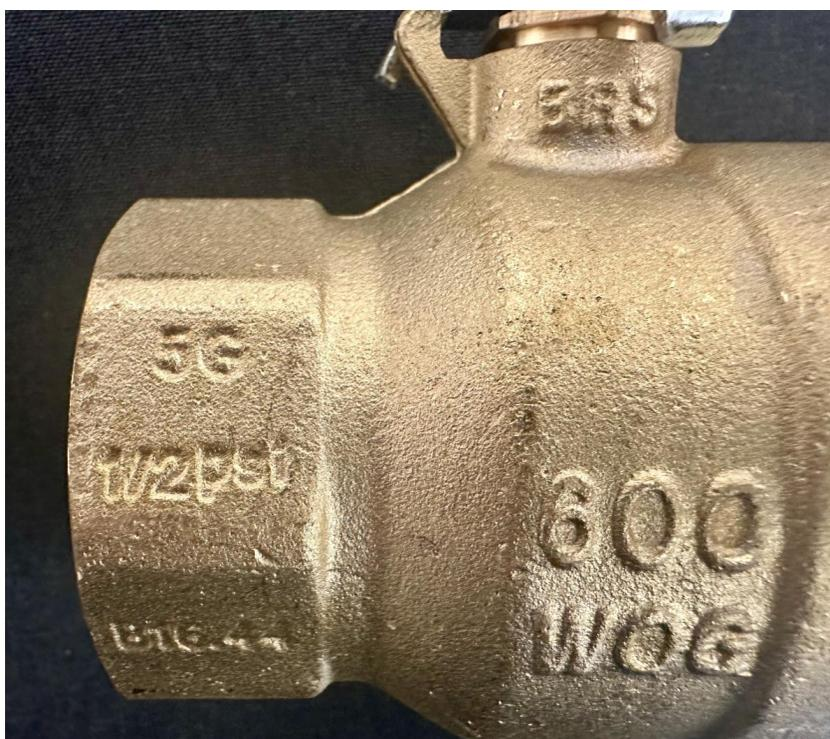
B16.44 does not apply to manually-operated gas valves which are an integral part of a gas appliance. These integral gas valves are subject to the *American National Standard for Manually Operated Gas Valves for Appliances, Appliance Connector Valves, and Hose End Valves, ANSI Z21.15/CGA 9.1* ANSI Z21.15 states that "A permanent marking specifying the maximum pressure rating of **1/2 PSIG** (3.5 KPa) shall be provided on each valve".
