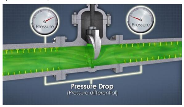
For our purposes today, pressure drop is calculated using a valve's Cv value. The Cv value, (also known as the Flow Coefficient), is the number of gallons of water per minute that can pass through a valve with a pressure drop of 1 psi. (Note: Pressure drop, \( \Delta P \), and differential pressure are all synonymous terms.) For example, on a 2-inch 509 check valve, the Cv from our spec sheet is 131.0. Therefore, this valve can pass 131 gallons per minute of water with a 1 psi drop.
