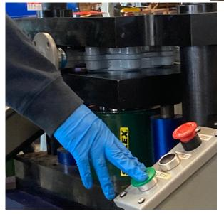
Both MSS and API require a shell test of 1.5x the CWP rating of the valve. In our example; 200 psig X 1.5 = 300 psig. So, that's the pressure to which Milwaukee Valve tests every valve rated to 200 psig.
