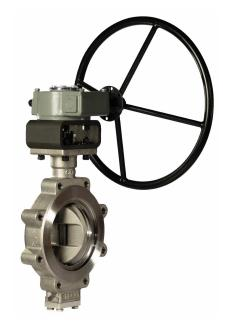
Triple offsets are generally used in applications where gate valves are found, where a metal seat is required, and tight shutoff and/or quarter-turn actuation is desired. Applications such as high-pressure steam (over 150 PSI), superheated-steam, high-temperature gases and oils, and other high-temperature applications are good for this type of valve. The triple offset valve is used in many similar industries as the double offset butterfly valve, but the applications are more demanding.
