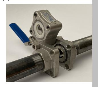
The choice between 2-piece and 3-piece is often based on the service. Some processes put heavy demands on valves, making a 3-piece valve more convenient for maintenance issues. If seats and seals need to be replaced, the 3-piece version allows for easy and routine disassembly, service and reassembly, without having to cut the valve out of the system. Three-piece ball valves also allow for elastomers to be changed to accommodate different process conditions, temperatures, pressures and flows.
