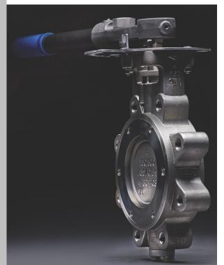
the characteristics of steam, if a disc is positioned less than 30 degrees open, it creates high velocity flow in the area between the disc and the seat. This high velocity steam can pull part of the seat out, which gets crinkled and damaged when the operator tries to close the valve.
