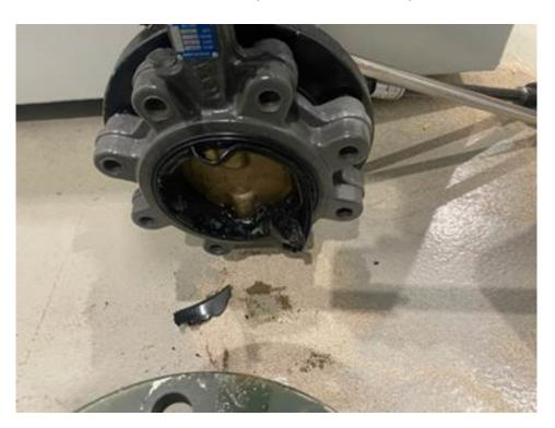
2. This valve was installed on a Purge Oil line. Purge Oil is used to preserve fuel tanks of jet aircraft when not in use for extended periods of time. Purge Oil is described as Petroleum Distillates, Hydrotreated Light, per the Material Safety Data Sheet (MSDS) that was supplied with the returned valve.
