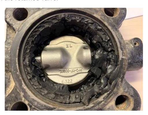
3. This valve was reportedly used on Jet A Fuel / Purge Oil. These are different media, so we're not sure which one did the damage. Regardless, EPDM would not be
