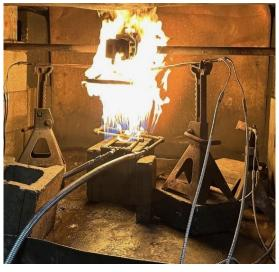
During fire testing, a pressurized closed valve filled with water is completely enveloped in high-temperature flames (around 750°C to 1000°C) for 30 minutes. The valve's ability to prevent leakage during and after the fire is measured to ensure it meets safety standards.
