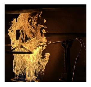
The American Petroleum Institute (API) has developed fire tests for valves used in the oil and gas industries. API 607 confirms the pressure-containing capability of quarter-turn valves under pressure during and after the fire test.
