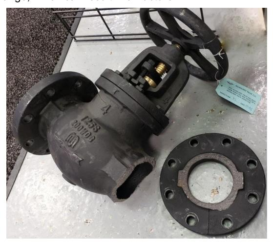
What does this mean for installers? Simply follow ASME guidelines – remove the raised face on the carbon steel flange and use a full face gasket. And while our first photo appears catastrophic, a worse scenario is a hairline crack and a leaking valve, which can do additional damage. At least the fracture is clear evidence that you have a problem, leading us to installation tip #2 today...
