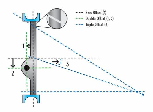
**Offset 1** – The stem is offset behind the seat axis, to provide complete sealing contact around the entire seat.
