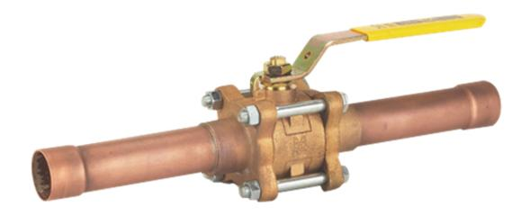
Milwaukee Valve's **BA-350TE** is designed for use in medical gas systems, pharmaceuticals and other applications where brazing or soldering is the preferred method of installation. This 3-piece bronze full-port ball valve includes 6" copper tube extensions brazed to each tailpiece. Because there is no need to disassemble the valve as required when installing other 3-piece valves, contractors can realize considerable labor savings with the **BA-350TE**.
