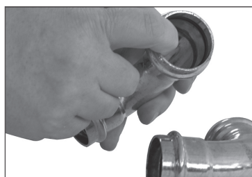
Figure 2: Check for EPDM Seal
