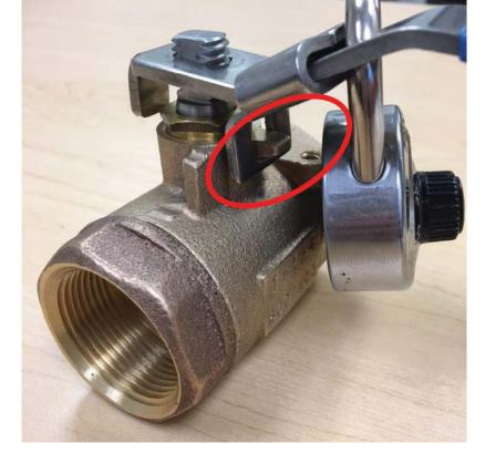
This shows the handle nut and lock washer removed, however, the handle is physically unable to be lifted off of the valve stem.
