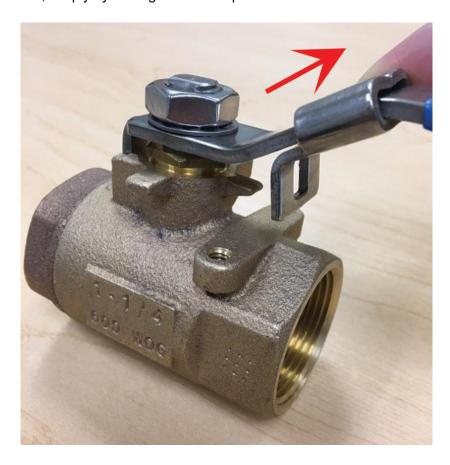
As depicted above, the collar needs to be moved up the handle to disengage the latch from the tab. The handle is then free to be turned 90 degrees.
