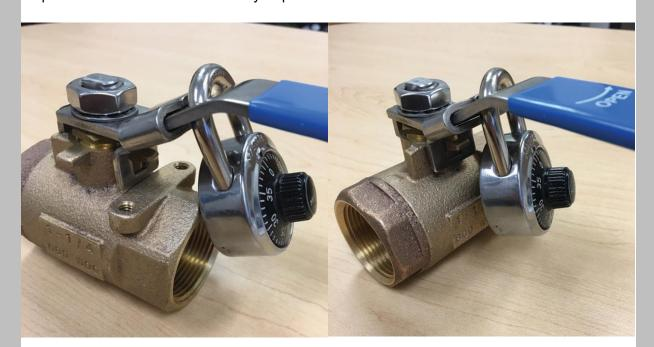
When the padlock is added, this collar cannot move to disengage the latch, thus locking the valve either open or closed, as seen above.
