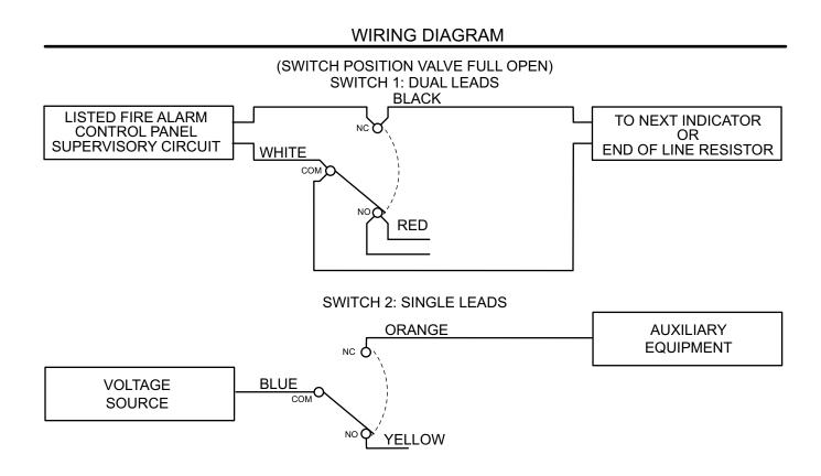
Green Lead provided is ground for switch housing Switch Rating: 10 AMP/115 VAC .5 AMP/28 VDC
