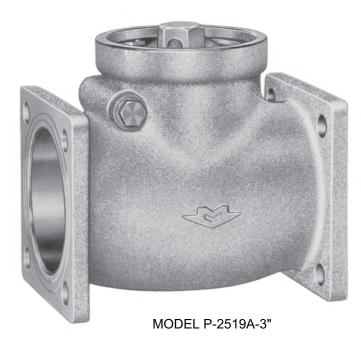
A rugged multi-purpose swing check for general tank and loading rack installations. All the advantages of full flow afforded by swing check design, near silent operation, leak resistance and quick cap removal; stainless steel pin and plugs.
