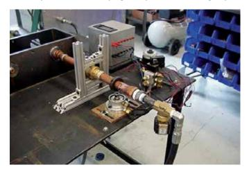
UltraPress® valves undergo a reverse bending/fatigue test, with superimposed alternating pressure spikes, to 250,000 cycles of bending with 250,000 [0-80-0] psig pressure cycles.
