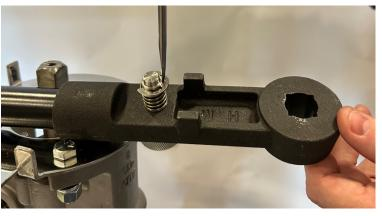
3. With the clip removed and the spring still on the Lock Knob, place the Lock Link (Larger Diameter Hole) over the Knob, compressing the spring down and reinsert clip into the groove of the Knob.
