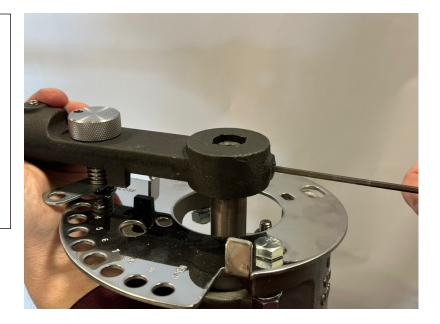
6. Add a padlock to prevent tampering with the disc fully open, fully closed, or in a throttling position.
