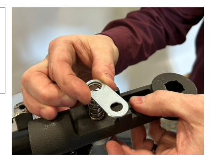
4. Reinstall Lever Handle onto the stem of the Valve. (Stem will **NOT** be flush with the top of the handle.)
