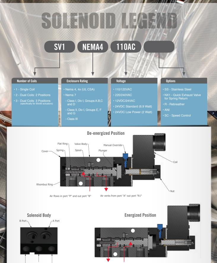
Exhaust Port R<sub>2</sub> Port P (Air In) Exhaust Port  $R_1$  Air vents from port "B" out port "R2"
