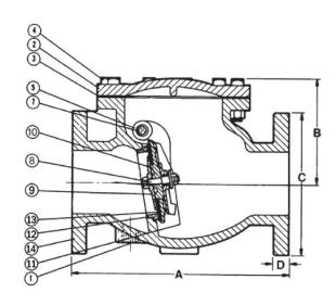
Note 1: On pump discharge, the preferred check valve is either an in-line spring loaded valve or a swing design with lever and weight. Install these valves as far as possible from the pump and elbows with a minimum distance of 5 times the pipe diameter.
