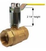
The -XLD extended locking handle is made of robust plated steel and provides additional safety benefits for the user. The handle can be locked in both the open and closed positions. Extension length provides for handle clearance above standard piping insulation thicknesses.
