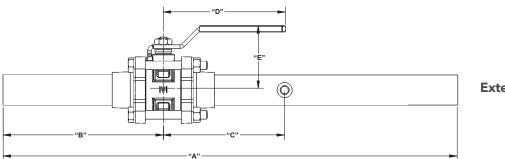
Bronze Ball Valve Three Piece Full Port 600 WOG Extended Tube Ends with 1/8" NPT Gauge Port Inline Repairable Blow-Out Proof Stem MSS SP-110
