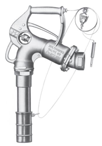
This easy-opening, soft-close valve minimizes shock. It is designed for operations up to 60 psi at inlet. Easy opening is achieved by balanced pressures on the valve assembly. Soft close controlled by balanced dashpot mechanism. Curved body minimizes friction and permits full flow. Poppet and dashpot assembly easily removed for repairs. Nozzle normally furnished with inlet adaptor, rigid tube, 100 mesh strainer, dust cap and ground cable. NPT inlet threads.
