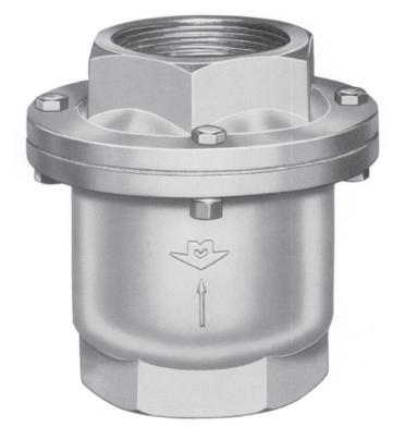
Vibration-proof disc construction, Viton-A\* renewable disc assures tight close at high temperature operation. Stainless poppet stem and disc retainer, guided top and bottom in friction free bushings.
