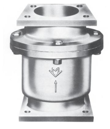
Vibration-proof disc construction, Viton-A\* renewable disc assures tight close at high temperature operation. Stainless poppet stem and disc retainer, guided top and bottom in friction-free bushings. Similar Lift Check with Quick Coupler Outlet is also available. For Threaded Version see P-728.
