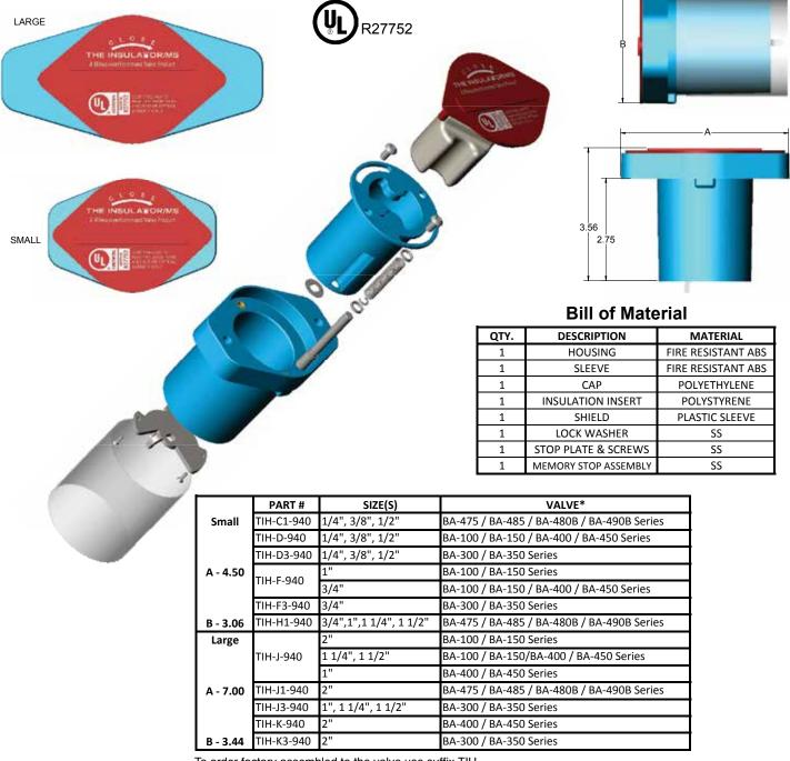
To order factory assembled to the valve use suffix TIH
