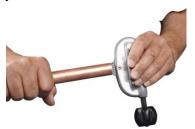
(1) The copper tubing should be cut square and the burrs, if any, should be removed with a file or scraper.
